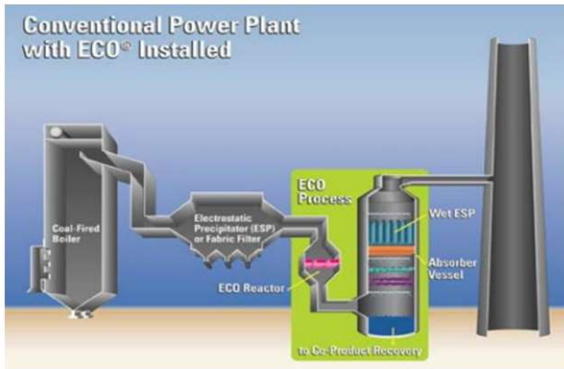
Typical ECO Installation Overview
