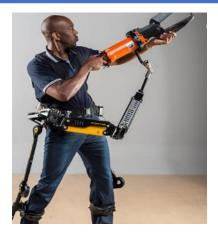
Designed to assist users in **holding, manipulating, and using heavy tools or** equipment.
